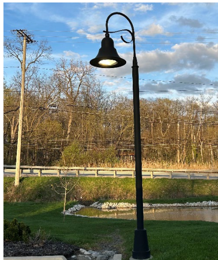
Figure 604-B – Cut-off light fixture example
